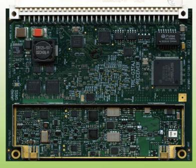
TRE-G3TAJT board also includes drivers for four LEDs, ON/OFF and function button controllers. In addition, the board comes with large amount of flash for data storage.
