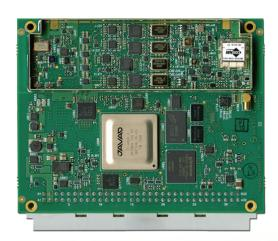
864 GNSS channels of this board allow tracking all current and future satellite signals. TRE-3N is form, pin-out, and command compatible with the TRE-3 and TRE-G3T boards.
