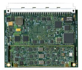
864 GNSS channels of this board allow tracking all current and future satellite signals. TRE-3 is the only receiver in the market that can track and decode the QZSS LEX signal messages. We offer highly stable digital filters (band characteristics do not change with age, input voltages, or temperature), improved GLONASS inter-channel bias performance (due to our flat digital filter shape), excellent new multipath rejection technique, the best ever.
